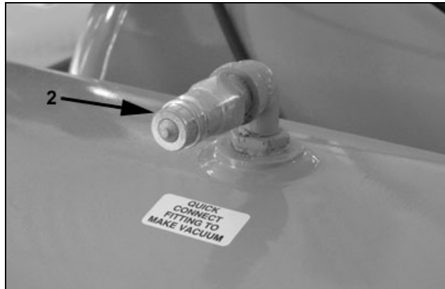
Figure 5 - Quick Disconnect Fitting to Make Vacuum
