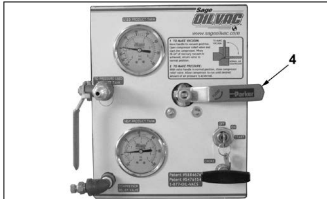
Figure 8 - 3-Way Valve in Air Compressor Position
