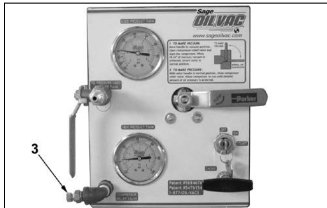
Figure 6 - Compressor Drain Valve
