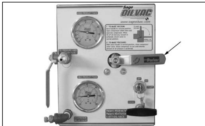
Figure 12 - 3-Way Valve in Air Compressor Position
