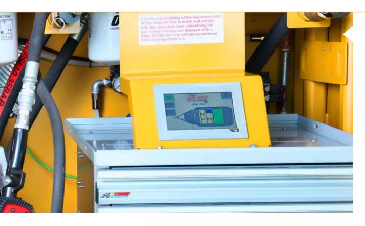
Technicians can view gallons within the tanks, instead of the percentage, making the process easier to determine the amount of oil available to complete an exchange.
