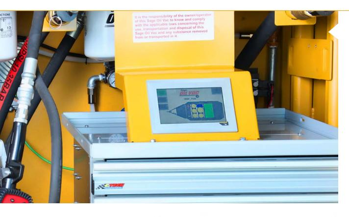
Technicians can view gallons within the tanks, instead of the percentage, making the process easier to determine the amount of oil available to complete an exchange.
